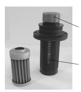
Breather with sealing disc and filter. Vents the tank if tankpressure > 10 mbar
